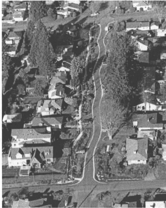
FIGURE 5-6 110<sup>th</sup> Street, Seattle, part of the Natural Drainage Systems Project. This location exhibits several elements of impervious cover reduction. In particular, vegetated swales were installed and curbs and gutters removed. There are sidewalks on only one side of the street, and they are separated from the road by the swales. The residences' rooftops have been disconnected from the storm-drain systems and are redirected into the swales. SOURCE: Seattle Public Utilities.
